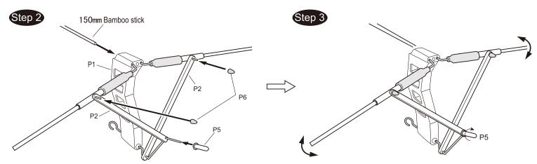
Cap and lock "P2" with 2 "P6"; Lock the other end of "P2" by pushing "P5" into the crank steel . Insert the 150mm bamboo stick into the hole on the other side of "P1" (sand the tip if needed )
