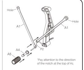
As the diagram shows, attach A1 to the bend in crank P2 of
