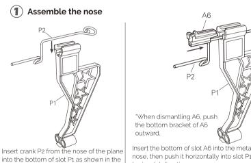
Insert the bottom of slot A6 into the metal wire of the nose, then push it horizontally into slot P1 in a horizontal direction.
